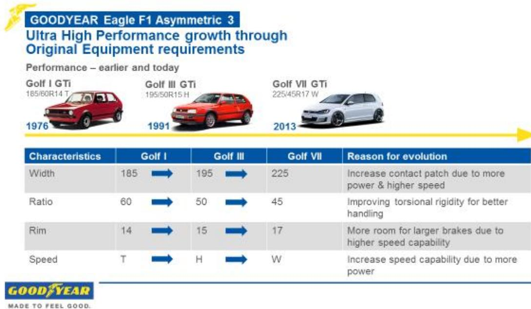
It is therefore to be expected that the number of tires coming from OE with higher speed ratings will increase, as small engine cars get higher horsepower due to advances in technology.
